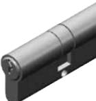
Another type of cylinder used with multi-point lock sets. These cylinders slip through the exterior escutcheon, the door and the interior escutcheon and are held in place by a set screw through the edge of the lock and vary in length for different door thicknesses.
