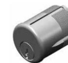
Mechanisms that are threaded into mortise locks, secured by a set screw through the edge of the lock and vary in length for different door thicknesses.
